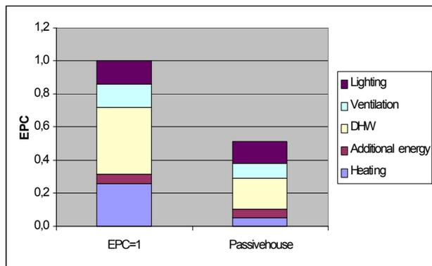
Fig. 1 Passive house versus modern Dutch standard houses
